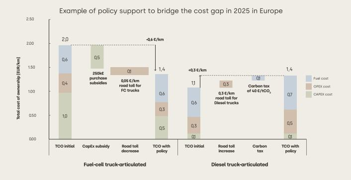
Figure 8: Policy support enabling the closing of the economic gap for fuel-cell articulated vehicles in the industrial scale-up phase (2030)
