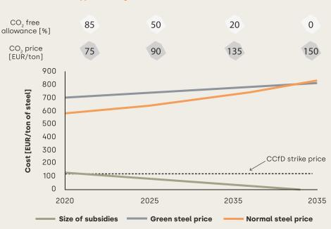
Figure 14: Illustration of a CCfD mechanism applied to the green steel market
