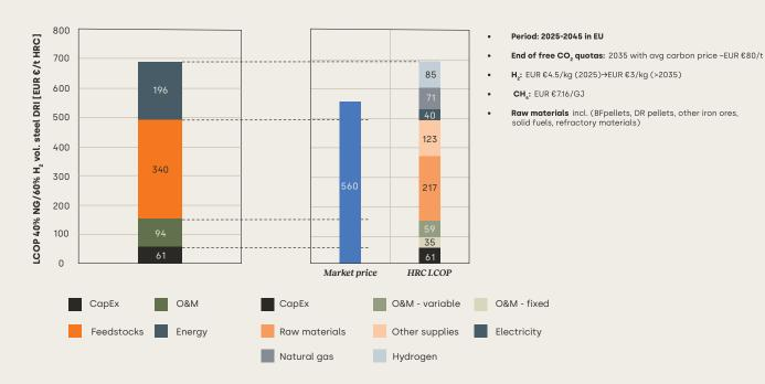
Figure 11 shows that OpEx represents over 90% of steel production costs. This underscores the significance of mechanisms that support OpEx, such as CfDs or CCfDs, as they offer promising avenues for cost optimization.
