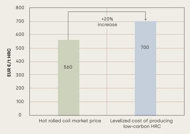
This cost difference arises from the higher capital expenditure of the DRI plant and the higher cost of energy (hydrogen and natural gas compared to coal) and feedstock (DRI pellets). Factors such as the additional infrastructure required, the availability and cost of hydrogen and the scale of production contribute to the higher cost of low-carbon steel than conventional steel produced using fossil fuels.
