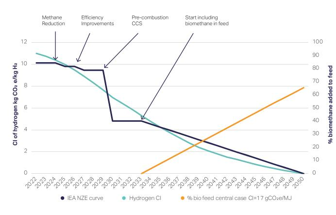
Figure 3: Example of an existing grey hydrogen project and its carbon intensity reduction
